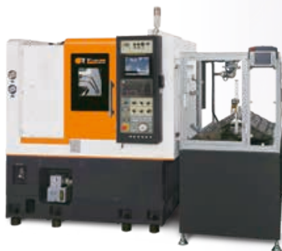
Vturn-NP16 with built-in robot
